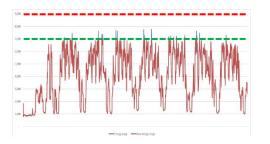
Use battery to reduce import from the grid during peak settlement periods, thereby reducing or eliminating grid charges that are linked to consumption during these periods
