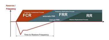
Use battery to offer various services to the national transmission network to help keep frequency balanced and ensure stability of the system
