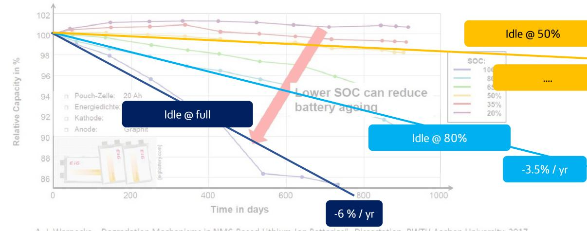
A. J. Warnecke, "Degradation Mechanisms in NMC-Based Lithium-Ion Batteries", Dissertation, RWTH Aachen University, 2017
